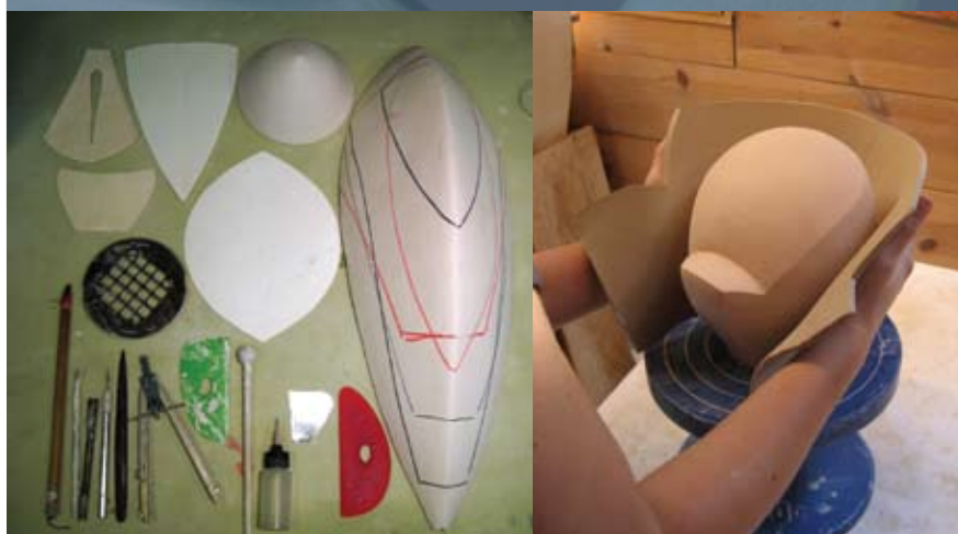
Clockwise from top left: spout patterns, two white teapot patterns, round bisque hump mold, large bisque hump mold with lines indicating placement of patterned slabs, Mudtool ribs (red and green), cut metal rib, underglaze applicator bottle, wooden stick with ball for smoothing hard-to-reach seams, compass for making patterns, black horn tool for smoothing, X-Acto knife for cutting smooth lines, hole cutting tool, scoring tool, paint brush.
